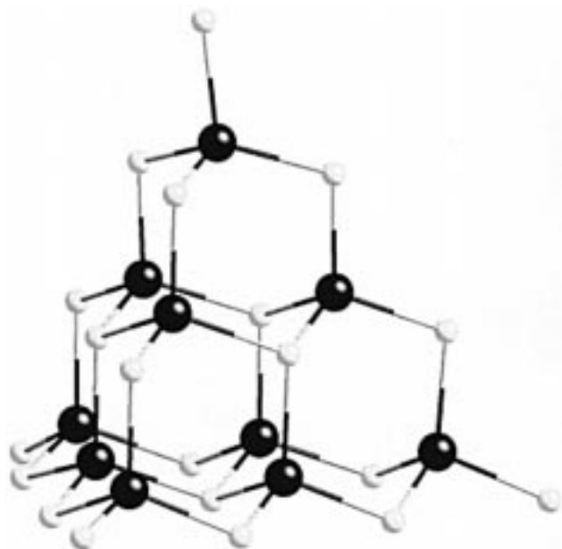
Figure 1. [\text{In}_{10}\text{S}_{20}]^{10-} supertetrahedron. Dark and light circles represent indium and sulfur atoms, respectively.
